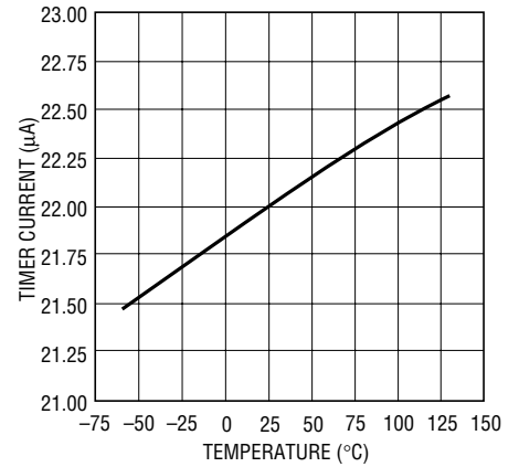
Timer Current vs Temperature
