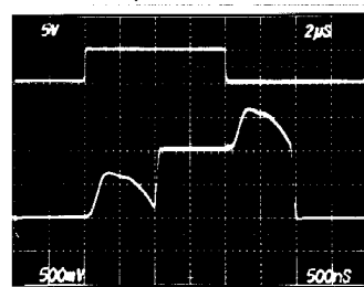
MUX-08 SMALL-SIGNAL SWITCHING WITH 2μs SAMPLE TIME
