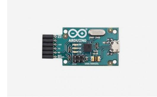
With the Arduino USB 2 Serial micro get the 5 volt TX and RX lines from a computer USB port that you can connect straight to the Arduino Mini 05 or to other microcontrollers for programming or data communication.
