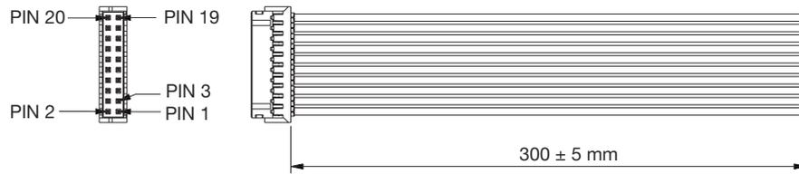
Order kit part number 73-788-001 for control connector interface with 0.3 m wires attached
