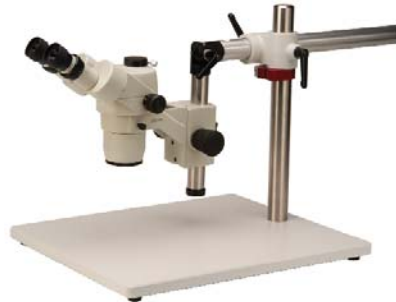
Binocular Scope on Single Arm Deluxe Stand with 17"x20" base
