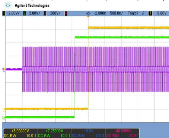
Figure 9: Turn-On AC Line 230 VAC, full load (5 ms/div)
