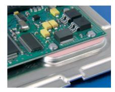
The true workhorse of the Sil-Pad product family, Sil-Pad 900S thermally conductive insulation material is designed for a wide variety of applications requiring high thermal performance and electrical isolation. These applications also typically have low mounting pressures for component clamping.
