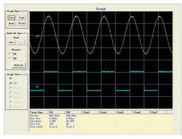
The included Easyscope software provides seamless integration between the oscilloscope and PC. Capture and transfer waveforms, screen images, setups and measurement results to a Windows PC via the USB device port on the back of the instrument.
