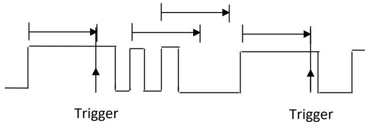
Figure 62 - State trigger
