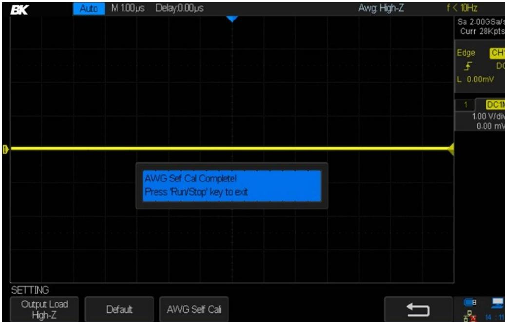
Figure 144 - AWG self-calibration
