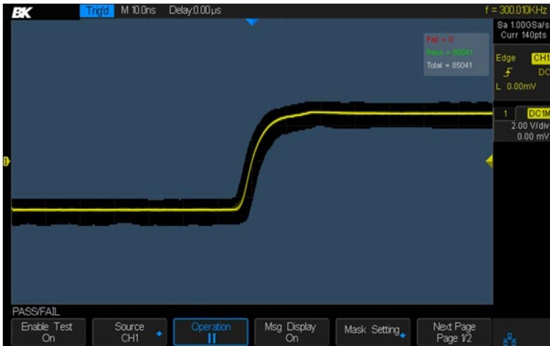
Figure 95 - Pass/Fail test
