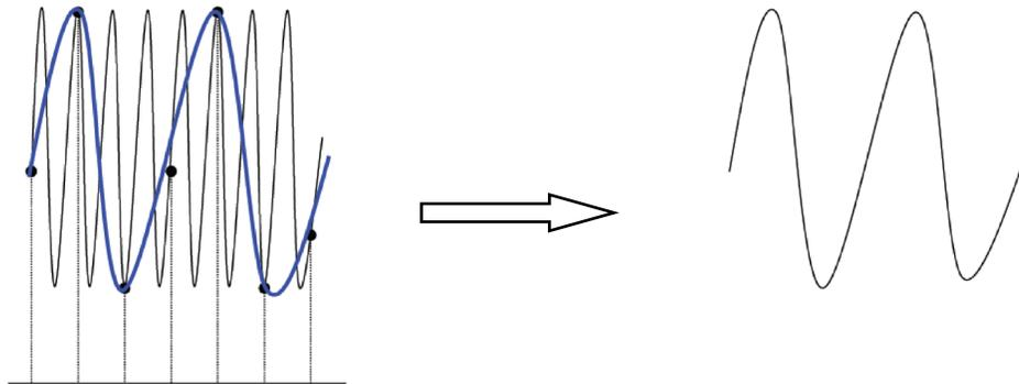
Figure 26 - Waveform aliasing
