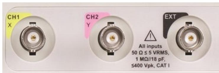
Figure 15 - Analog and external trigger connectors
