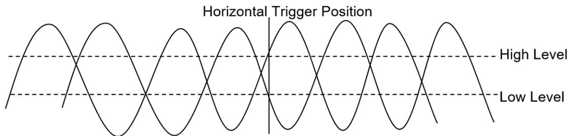
Figure 55 - Window trigger
