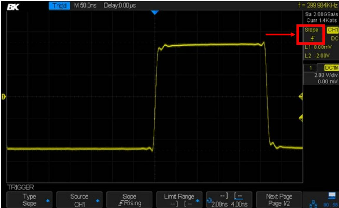
Figure 51 - Slope trigger
