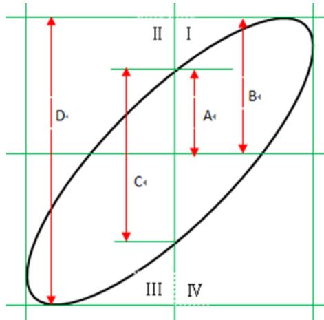
Figure 39 - Calculating phase difference with Lissajous figure
