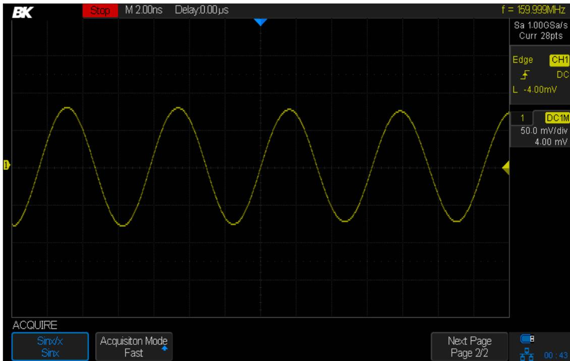
Figure 32 - Sinx/x interpolation
