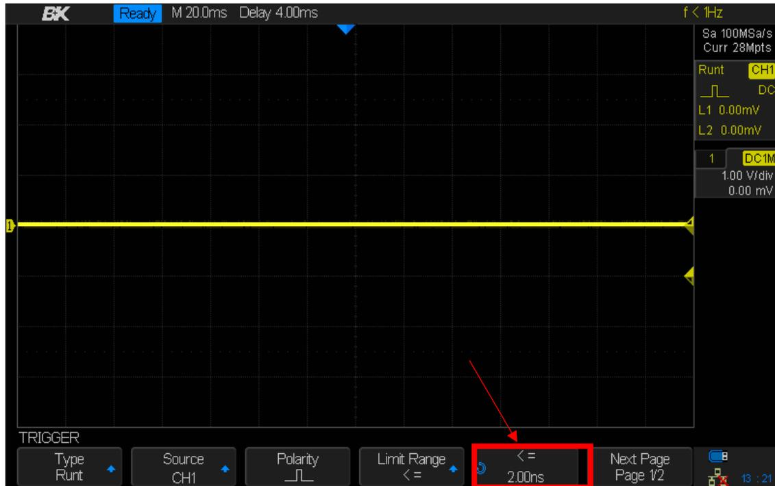
Figure 65 - Time setting runt trigger
