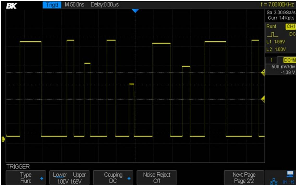
Figure 66 - Runt trigger
