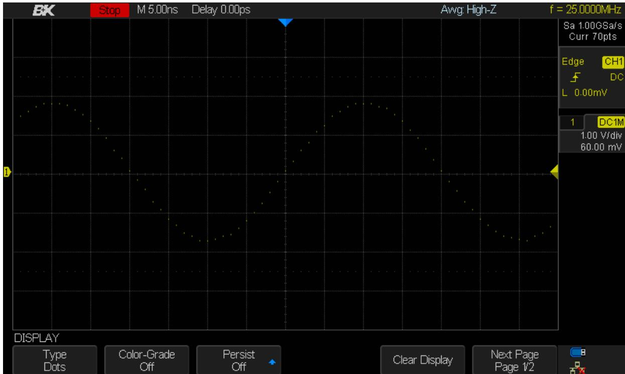
Figure 89 - Dots display
