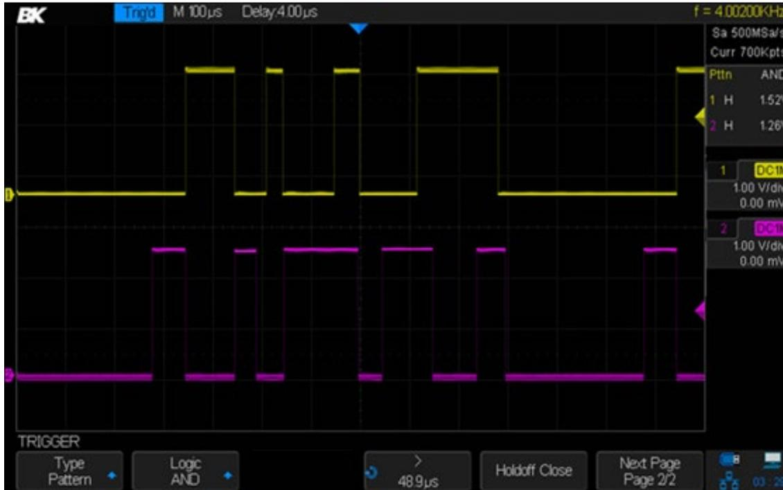
Figure 68 - Pattern trigger
