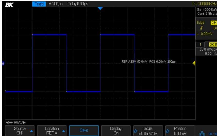
Figure 104 - Reference waveform
