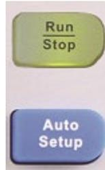
Figure 22 - Run control buttons
