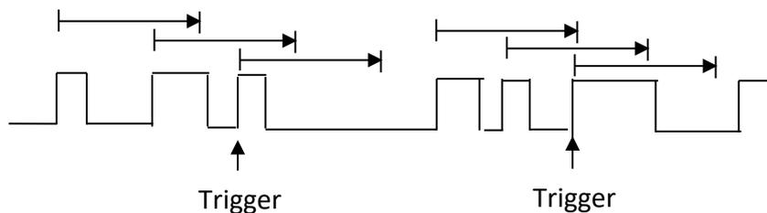
Figure 58 - Interval trigger
