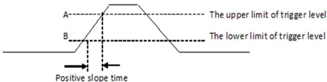
Figure 50 - Positive slope time
