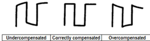
Figure 12 - Waveform compensation
