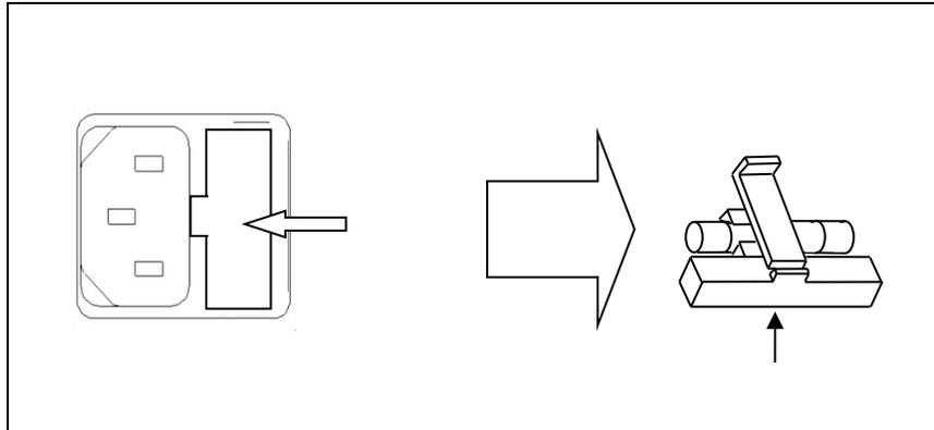
Figure 7 - Replacing Fuse
