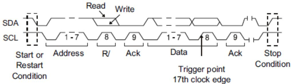
Figure 71 - 7-bit address and data condition trigger (17<sup>th</sup> clock edge)
