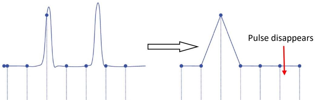
Figure 27 - Waveform leakage
