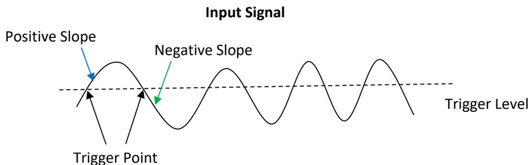
Figure 44 - Trigger level for an edge trigger
