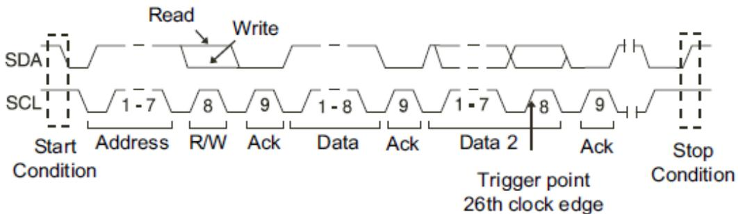
Figure 72 - 7-bit address and data condition trigger (26<sup>th</sup> clock edge)
