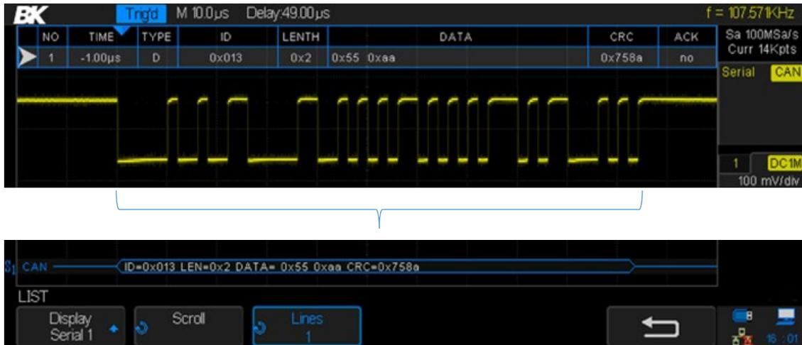
Figure 121 -CAN Decode
