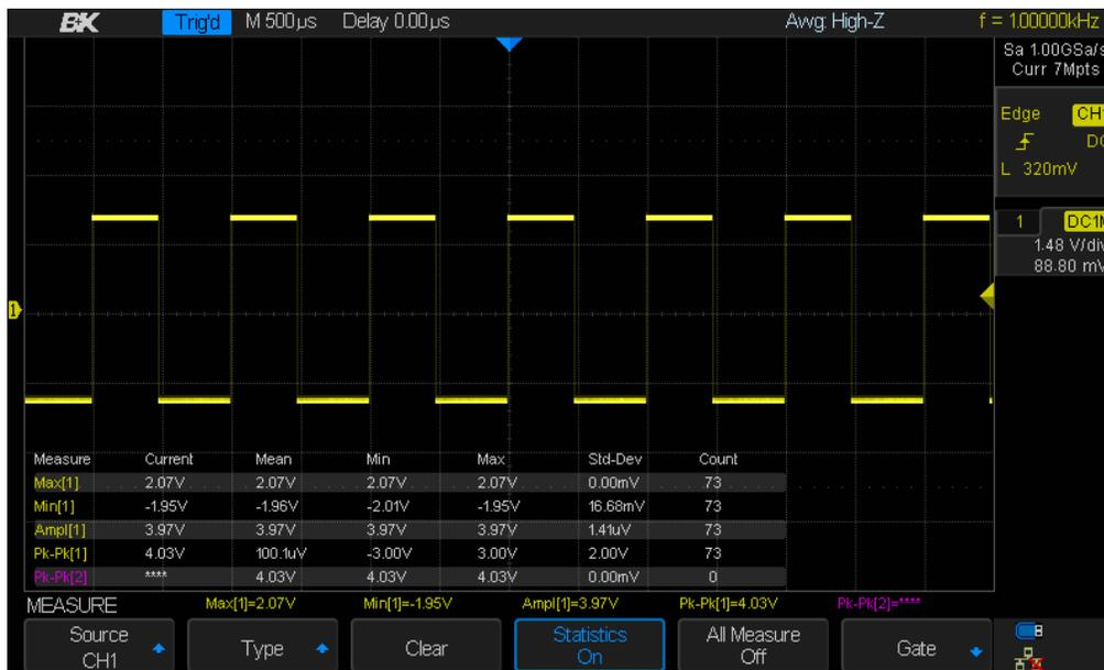
Figure 86 - Selected measurements and the table of statistics
