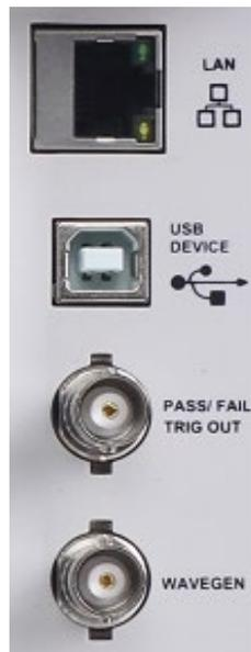
**Figure 18 - Rear panel connectors**
