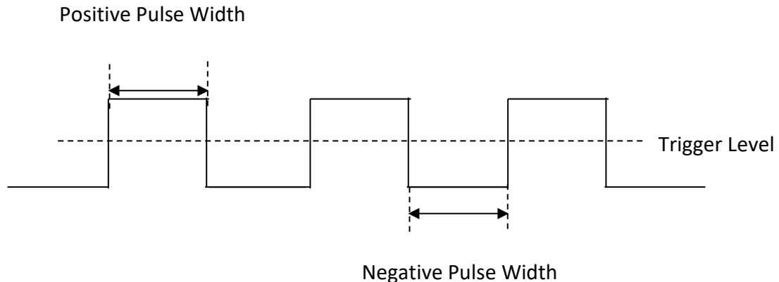
**Figure 52 - Pulse Trigger**
