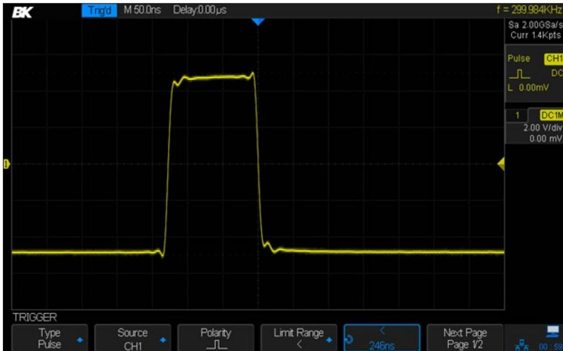
Figure 53 - Pulse trigger
