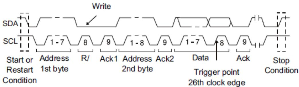
Figure 73 - 10-bit address & data condition
