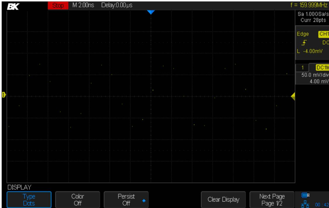
Figure 30 - Display type set to dots
