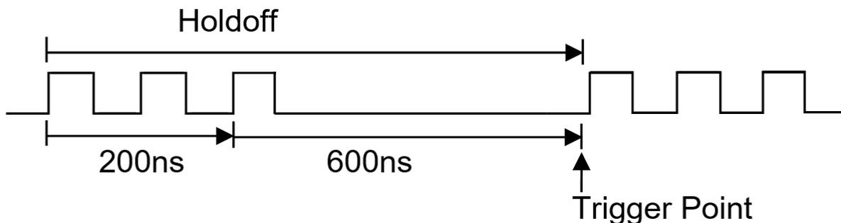
Figure 45 - Trigger hold off
