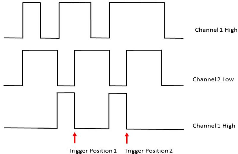
Figure 67 - Pattern Trigger
