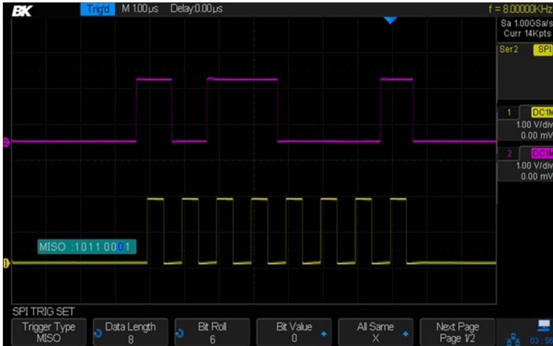
Figure 75 - SPI trigger
