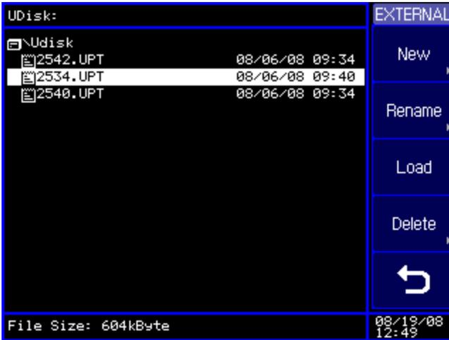
Press the **Load** softkey to start the update operation. A loading progress bar and then an updating progress bar will be displayed and indicate the progress of the update operation.
