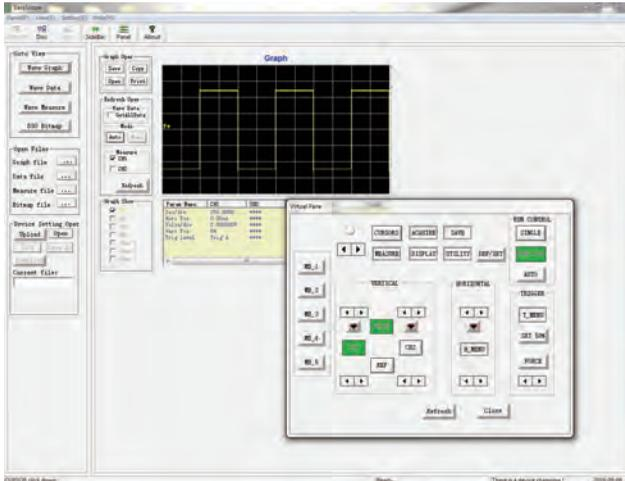
The included EasyScope software provides seamless integration between the oscilloscope and PC. Capture and transfer waveforms, screen images, setups and measurement results to a Windows PC via the USB device port on the back of the instrument. A USB host port on the front and rear allows for quick and easy screen saving.
