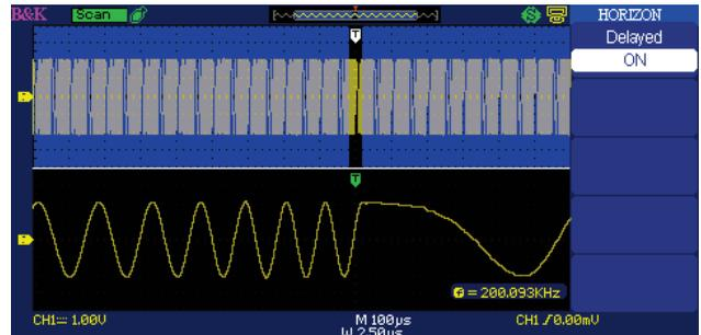
Use the oscilloscope's delayed sweep feature to zoom in a particular area of a signal in real time while viewing the entire captured waveform simultaneously.
