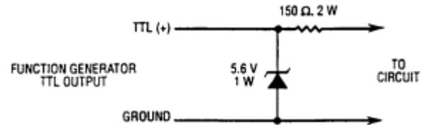
**Figure 7. Circuit for Protection of TTL Output.**
