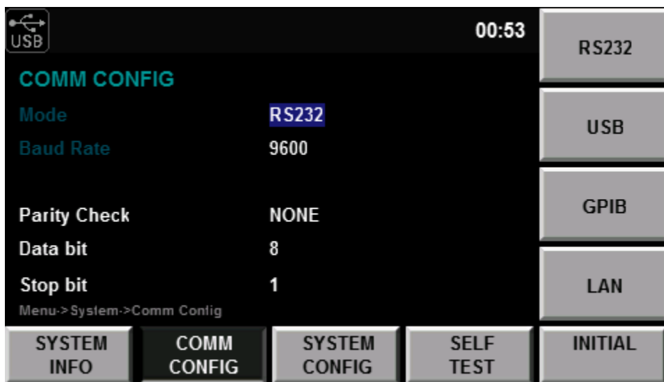
Figure 2.3 COMM Configuration - RS-232
