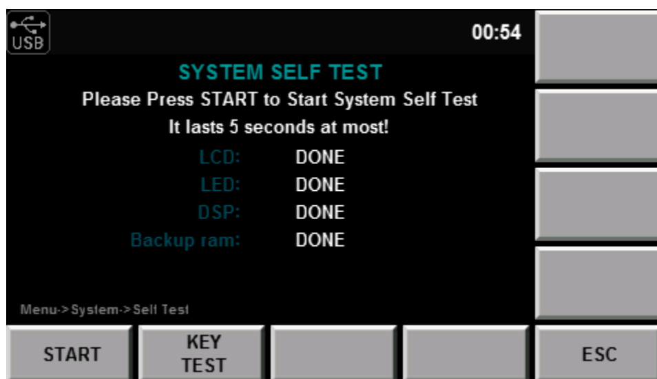
Figure 2.9 System Self Test
