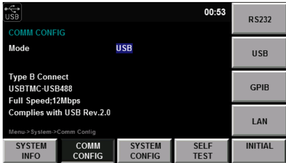
Figure 2.4 COMM Configuration - USB
