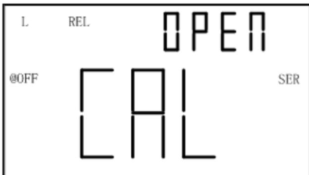
**Figure 7 - Open Calibration**
