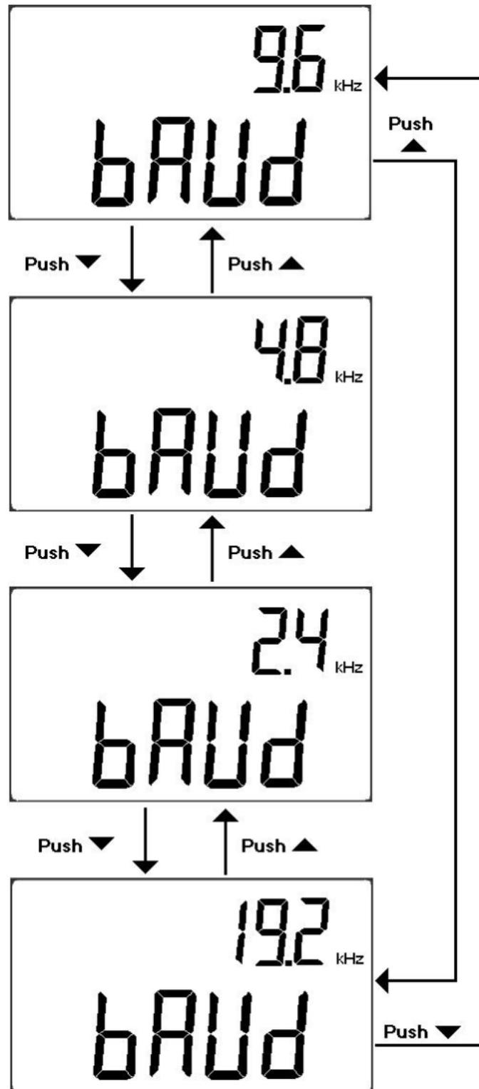
Figure- 5 Baud rate setup for remote control
