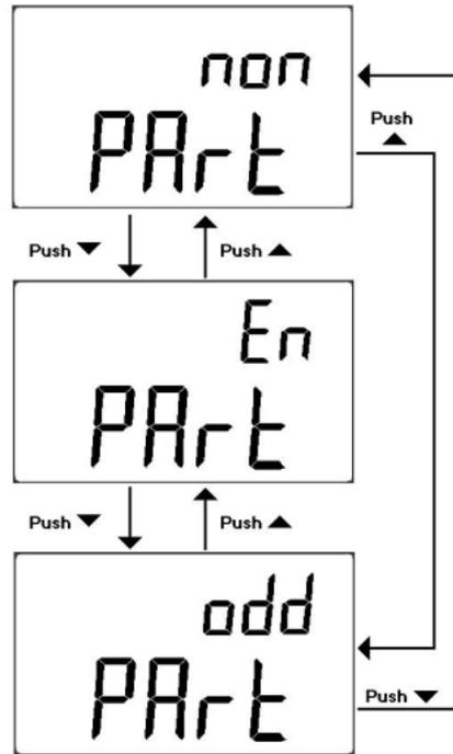
Figure- 6 Parity Check setup for remote control
