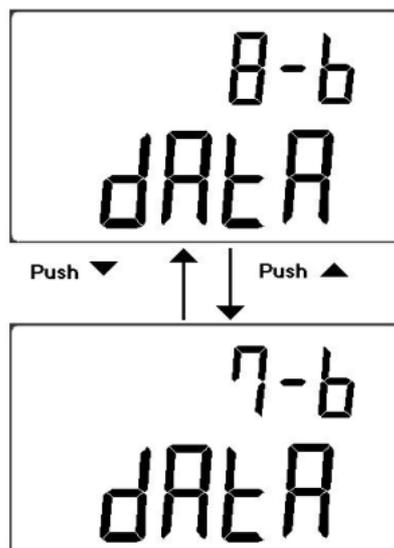
Figure- 7 Data bit setup for remote control
