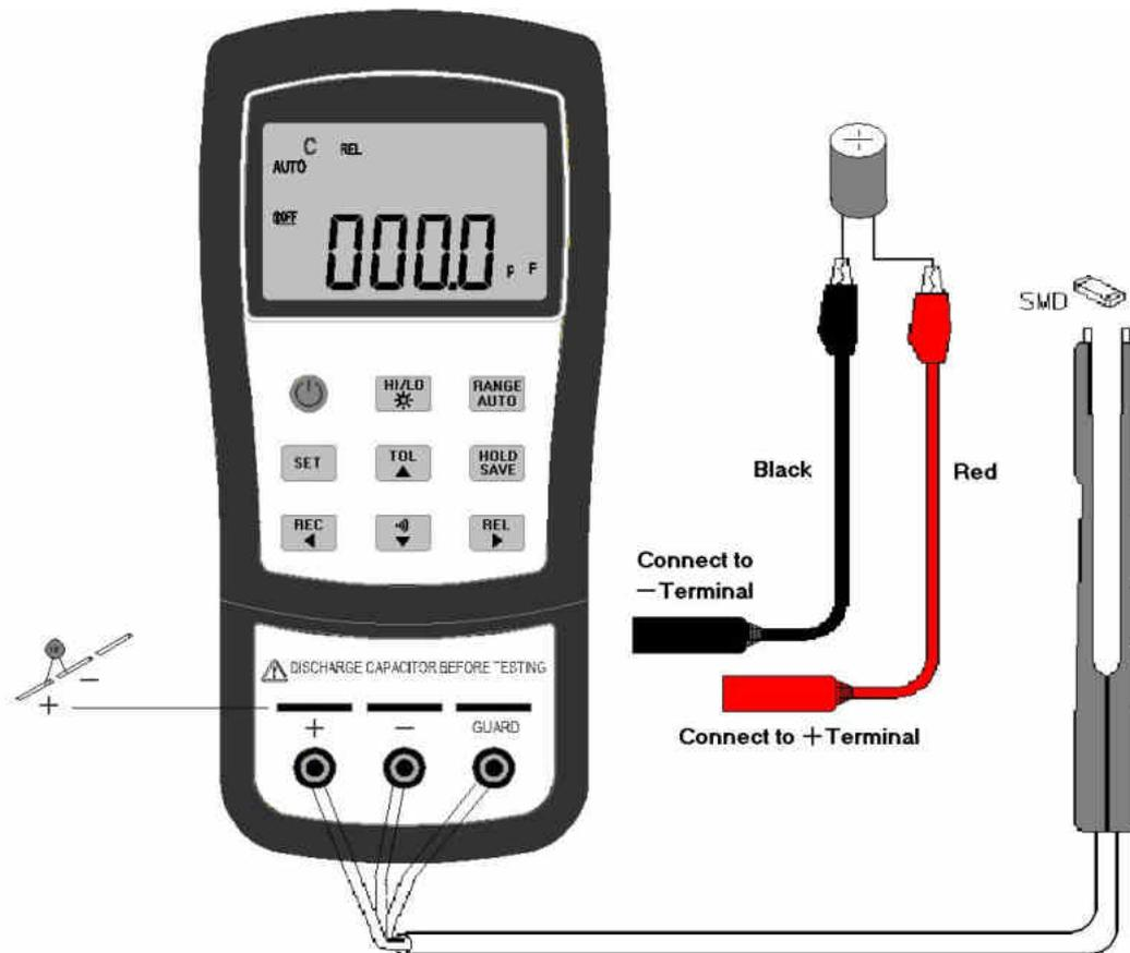
Figure- 25 Capacitance measurement
