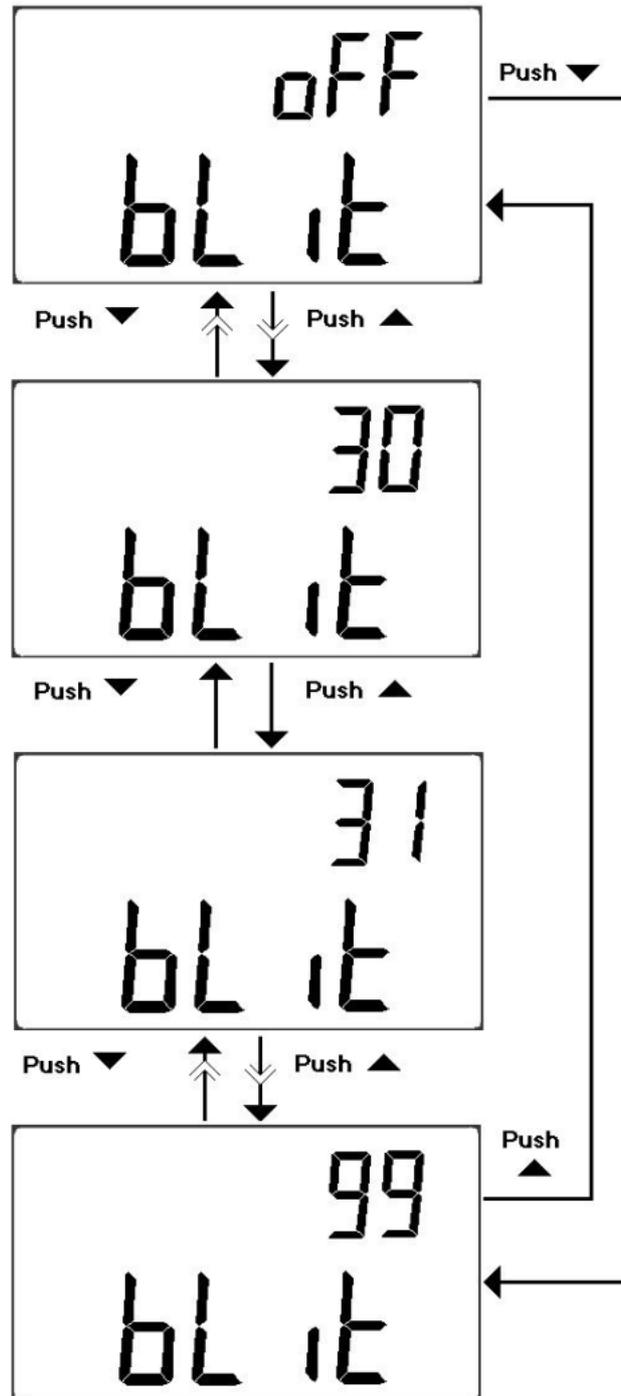
Figure- 13 Backlit Timer Setup
