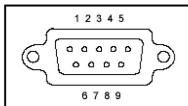
The DB9 connector in the rear panel of the power supply provides a TTL level signal. It can be connected to a standard PC interface via the IT-E131 or IT-E132 isolated communication cable.
