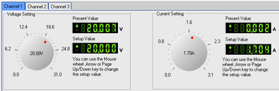
Use the mouse to click on the rotary knob and move the mouse to change the value. You also can use the mouse wheel, or Page Up/Down keys and arrow keys (↑, ↓, ←, →) from the keyboard for fine adjustment of voltage or current values.. The setup value will be displayed on the second line indicator.
