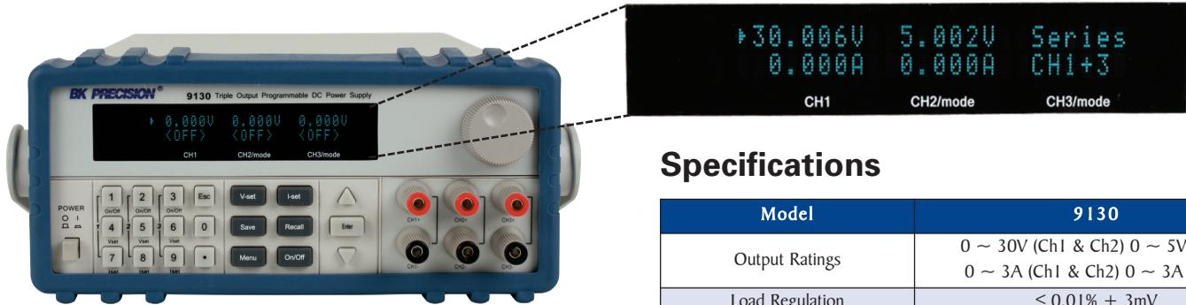
The 9130 is a fully programmable triple Output DC Power Supply delivering 0-30V/0-3A on 2 outputs and 0-5V/0-3A on 1 output. Each output is fully floating and outputs can be adjusted independently or connected in series or parallel to produce higher voltages or currents. The 9130 is ideally suited for applications in Electronic Test, Production and Service where multiple independent DC supplies are required and bench space is at a premium.
