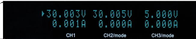
The 9130 is a fully programmable triple Output DC Power Supply delivering 0-30V/0-3A on 2 outputs and 0-5V/0-3A on 1 output. Each output is fully floating and outputs can be adjusted independently or connected in series or parallel to produce higher voltages or currents. The 9130 is ideally suited for applications in Electronic Test, Production and Service where multiple independent DC supplies are required and bench space is at a premium.
