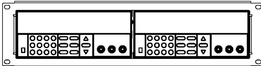
To rack mount two instruments side-by-side, order rack mount kit IT-E151, you needn't to use the front cover panel.
