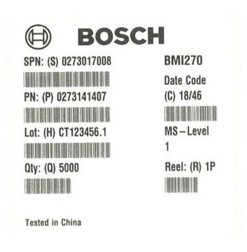
The dimensions of the bar code label are approximately 61 mm x 74 mm.
