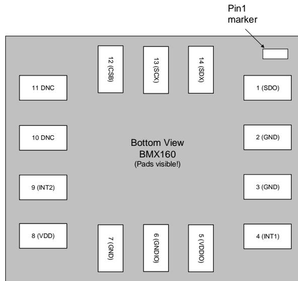
Figure 31: Pin-out bottom view
