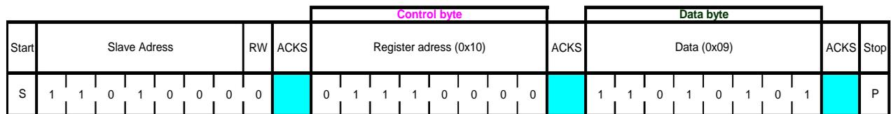
Figure 28: I<sup>2</sup>C write
