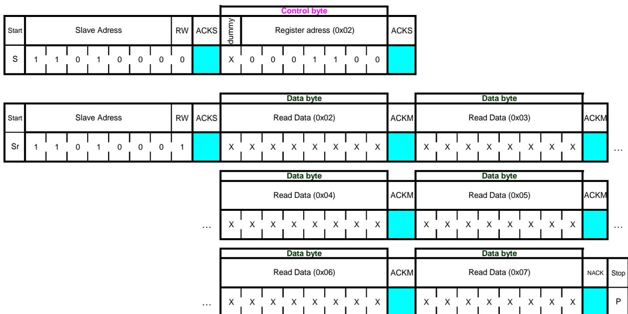
Figure 29: I<sup>2</sup>C multiple read
