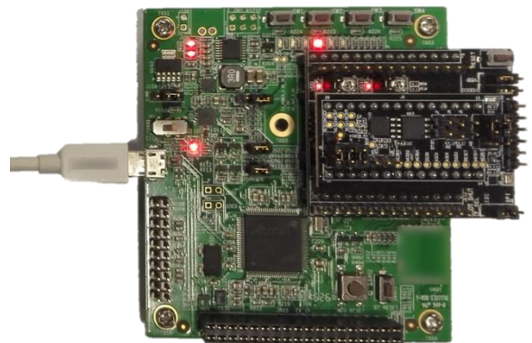
Connection of shuttle board, level shifter board and application board
