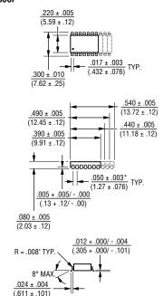
Lead coplanarity .004 inch max. at mounting surface.
