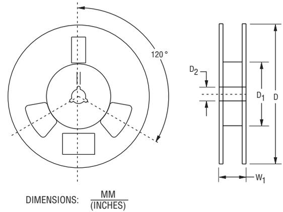
Devices are packed in accordance with EIA standard RS-481-A.
