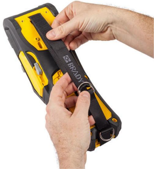
7. Slip your hand through the strap to provide a secure grip when holding the printer.
