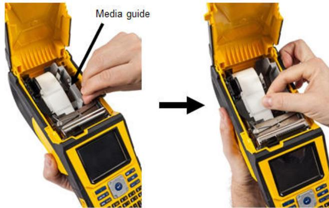
5. With the Power on, press Feed button once to feed media under printhead.
