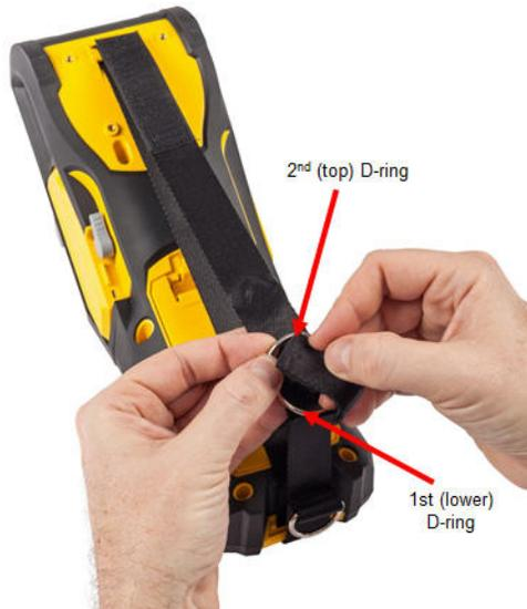
6. Pull the loose end of the strap until it feels tight, then press the scratch (burr) fastener against the strap so it lays flat.
