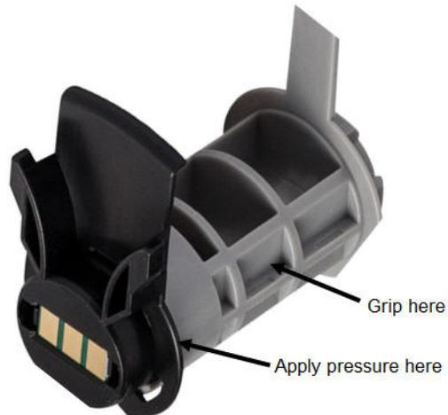
4. From the back side of the black end cap, press the blade of the screwdriver against the locking tabs, applying outward pressure. This will release the smart cell.
