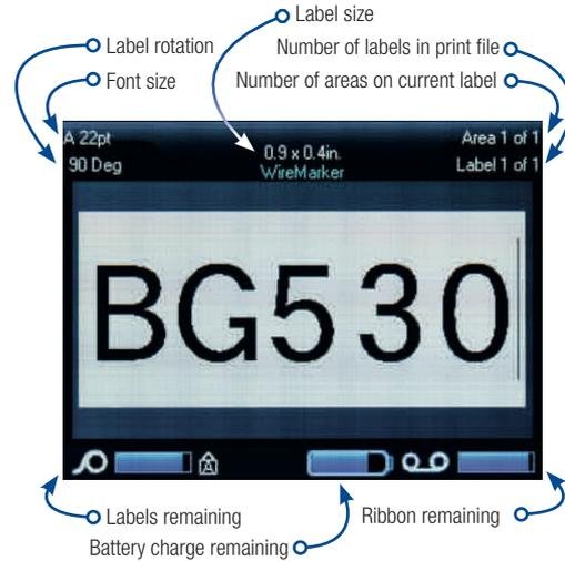
Every BMP61 label and ribbon is automatically recognised and auto-calibrated by the printer. The printer's colour touch screen displays which label material is currently installed and how many labels, how much ink and how much battery is left for maximum ease of use.
