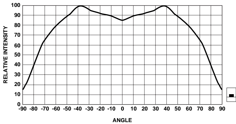
Figure 6. Relative intensity vs. angle for HSMx-C120.
