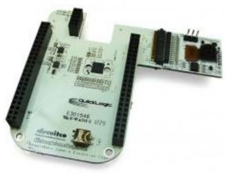
Note: BeagleBone 3.1MP Camera Cape should be used with LCD7 Cape or DVI-D Cape for previewing and capturing photos.
