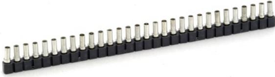
Part number MS11 consists of a carrier strip of 30 cage jacks. The strip can easily be cut to any desired number of cage jacks. These are mounted directly in a print circuit board. After soldering, the carrier is pulled off the cage jacks. Use a spacer between the PCB and the heatsink to avoid short circuits.
