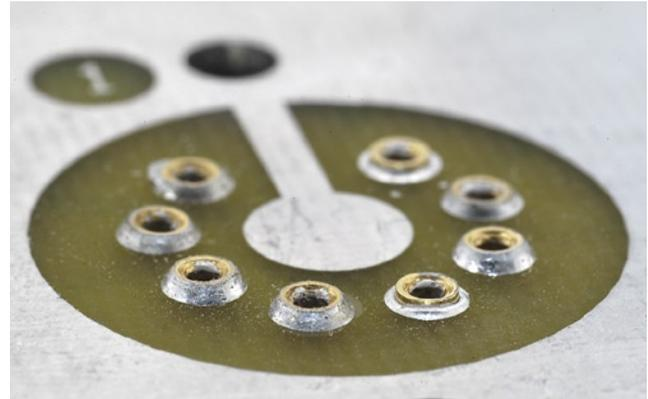
Part number MS02 consists of a package of 8 cage jacks. These are mounted directly in a print circuit board. Use a spacer between the PCB and the heatsink to avoid short circuits.
