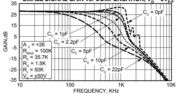
**SMALL SIGNAL GAIN vs. COMPENSATION,  $V_o = 500mV_{P-P}$**
