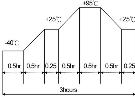
The diagram illustrates a temperature cycle over a 3-hour period. It starts at  $-40^{\circ}\text{C}$  for 0.5hr, ramps up to  $+25^{\circ}\text{C}$  in 0.5hr, dwells at  $+25^{\circ}\text{C}$  for 0.25hr, ramps up to  $+95^{\circ}\text{C}$  in 0.5hr, dwells at  $+95^{\circ}\text{C}$  for 0.5hr, ramps down to  $+25^{\circ}\text{C}$  in 0.5hr, and dwells at  $+25^{\circ}\text{C}$  for 0.25hr. The total cycle time is 3 hours.
