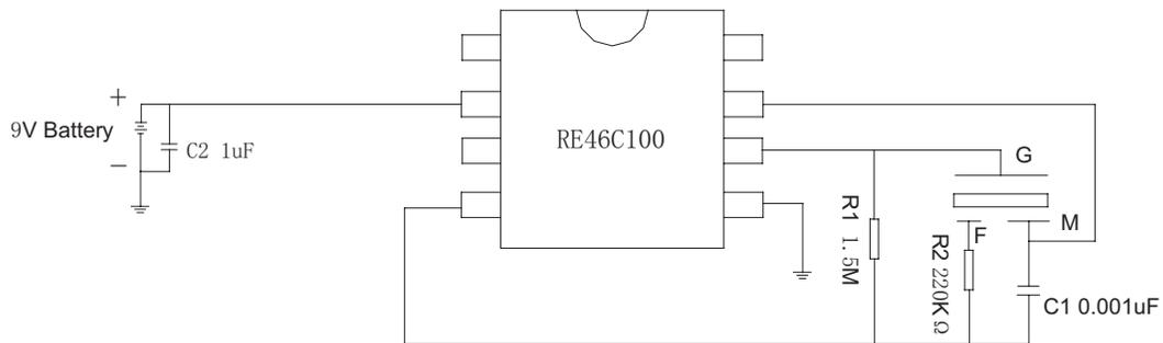
Notes: 1. The current consumption and the sound pressure level are measured by using the recommended driving circuit shown above.
