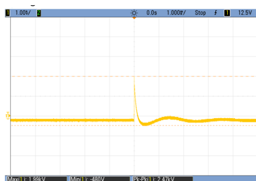
Input voltage waveform (Differential mode 1.99KV)
