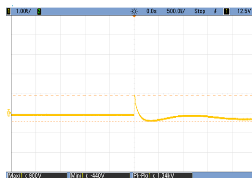
Output voltage waveform (0.9 KV)
