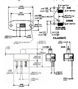
NOTE: SPST versions have one end terminal (shown in blue) removed. Provision for varying current and voltage rating is made by changing internal contact materials.
