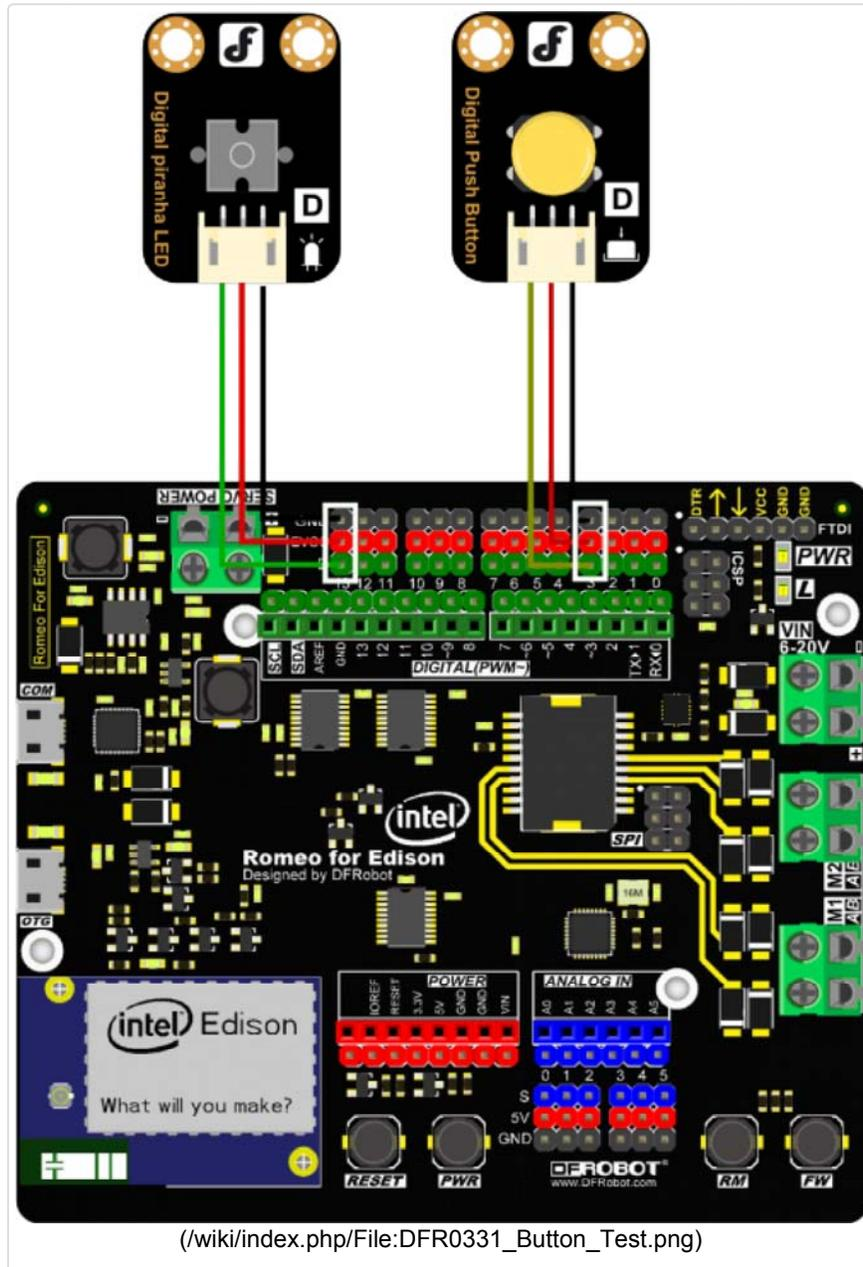
Sample code: Open Arduino IDE, Select Boards --> Intel Edison and COM port
