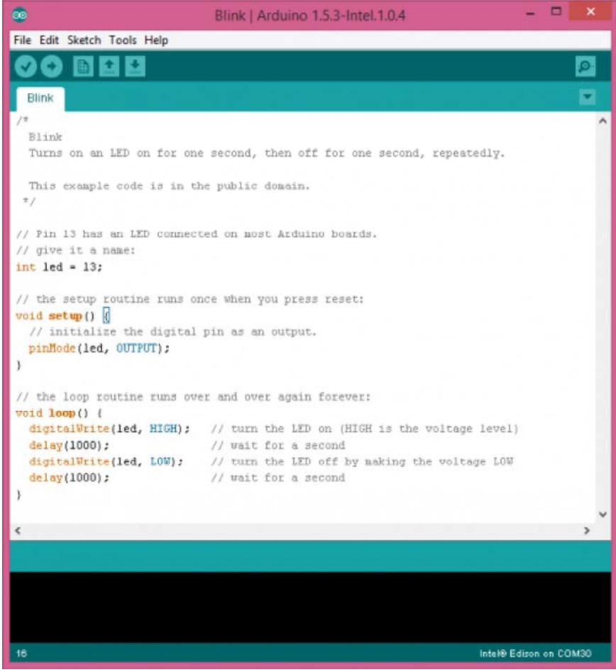
The image shows a screenshot of the Arduino IDE interface. The title bar reads "Blink | Arduino 1.5.3-Intel.1.0.4". The menu bar includes "File", "Edit", "Sketch", "Tools", and "Help". Below the menu bar is a toolbar with icons for saving, opening, and other functions. The main text area contains the following code:
