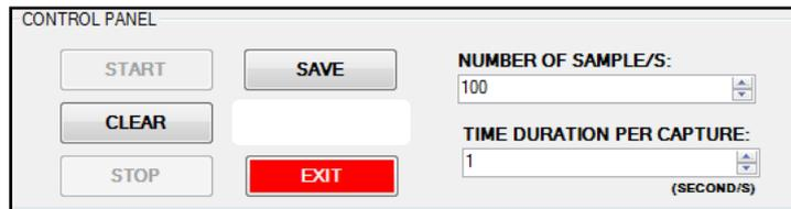
To start the data logging, select the number of samples by pressing the up down arrow. Next, select the time duration per capture according. Click START button to initiate data logging. Click STOP button to halt data logging and click CLEAR button to erase or click SAVE button to store the data. EXIT button is used for quit Single Angle Graph window.
