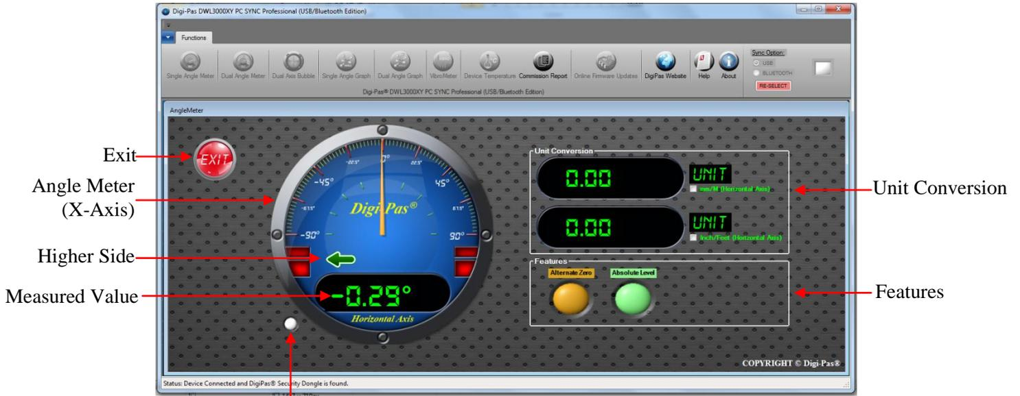
Blinking indicates measurement is in progress
