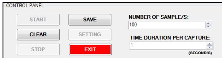
To start data logging, select the number of samples by pressing the up down arrow. Next, select the time duration per capture accordingly. Click START button to initiate data logging. Click STOP button to halt data logging and click CLEAR button to erase or click SAVE button to store the data. The SETTING button can be used to configure the row visibility window of the recorded data. EXIT button is used to quit the Dual Axis Bubble window.
