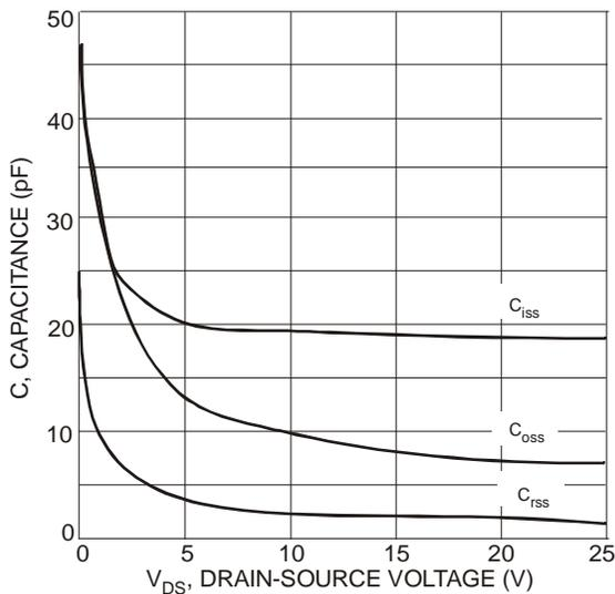
Fig. 5 Typical Capacitance
