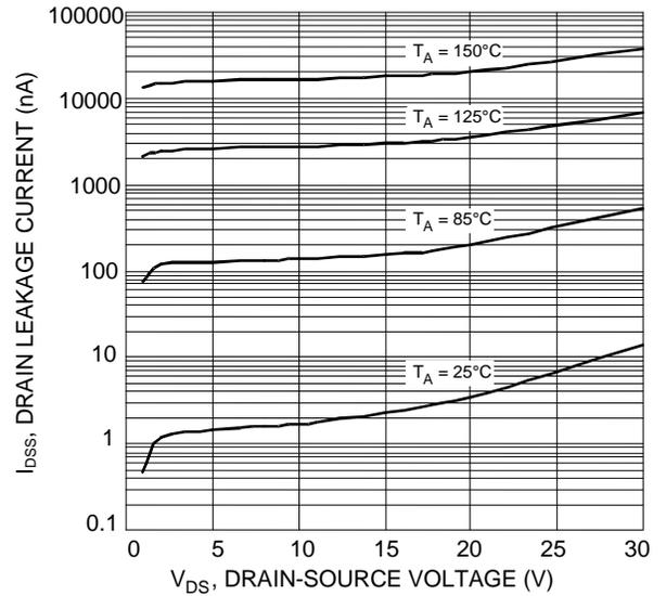
Figure 10 Typical Drain-Source Leakage Current vs. Voltage
