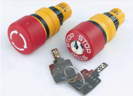
Emergency-stop, twist release and key release, 27mm diameter for 16mm mounting, foolproof to EN 60947-5-5 and EN 418
