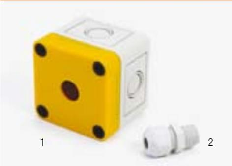
Emergency-stop switch enclosure with 16 mm mounting hole, 65 mm (w) x 65 mm (h) x 57 mm (d) and cable gland M16, IP66
