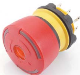
Emergency-stop red LED illuminated, plug-in terminals, twist release, 32mm diameter for 22.5mm mounting, foolproof to EN 60947-5-5
