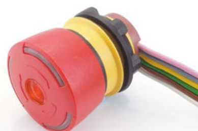
Emergency-stop red LED illuminated, ribbon cable, twist release, 32mm diameter for 22.5mm mounting, foolproof to EN 60947-5-5
