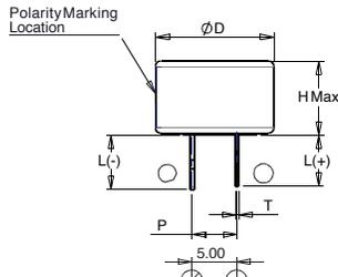
Recommended PCB Layout  $\varnothing 1.60 \pm 0.05$
