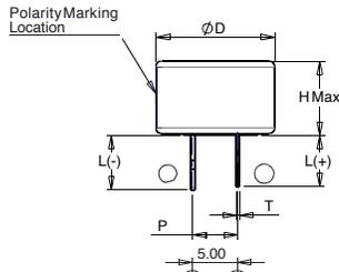
Recommended PCB Layout  $\text{Ø}1.60 \pm 0.05$
