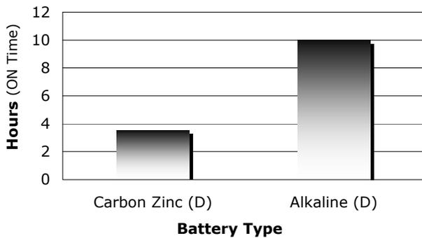
**Typical Battery Service to 0.9V (per battery) at 21°C (70°F)**
