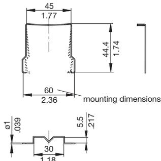
**Retaining clip for circuit breaker 2210**
