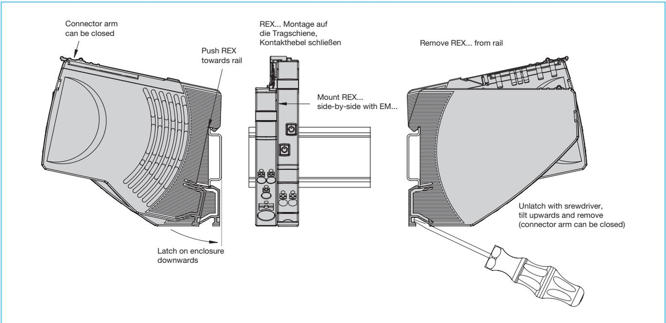
Application example: REX... Replacement or disassembly
