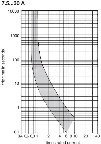
The time/current characteristic curve depends on the ambient temperature prevailing. In order to eliminate nuisance tripping, please multiply the circuit breaker current ratings by the derating factor shown below. See also section Technical information.
