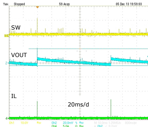
Fig. 7: V_{OUT} ripple is 22mV at 0A, DCM, 12VIN, 1.2VOUT
