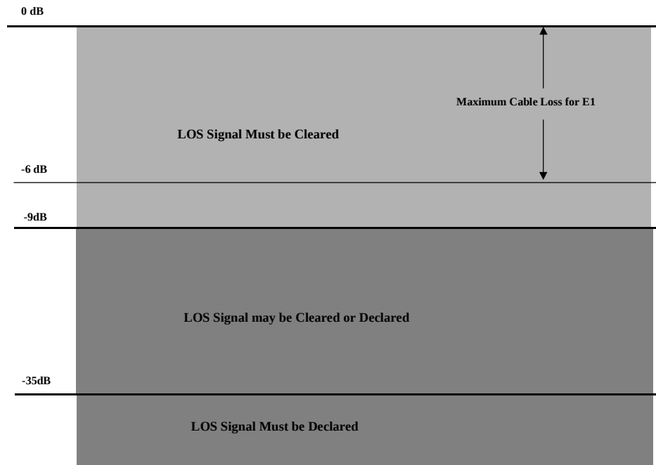
Figure 10. Illustration of the Signal Levels that the Receiver Sections (within XRT5997 device) will declare and clear LOS
